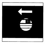
To do so, slide the unlocking switch (10) at the forward right of your balance in the arrow direction.
