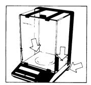
At the point of use, level the balance using the leveling screws (6) such that the air bubble is centered in the circle of the level indicator (5).
