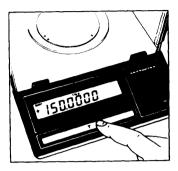
Clear the pan and depress the tare button for at least three seconds until the calibration weight appears in the display.
