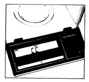
After a few seconds, the display will read "CC", followed by 0.0000 g. A beeper confirms successful completion of calibration.
