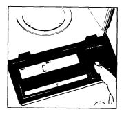
Clear the pan and zero the display. Once the display reads 0.0000 g, push the CAL button (8). The display now reads "C". If you get "CE", zero the display and push the CAL button again.
